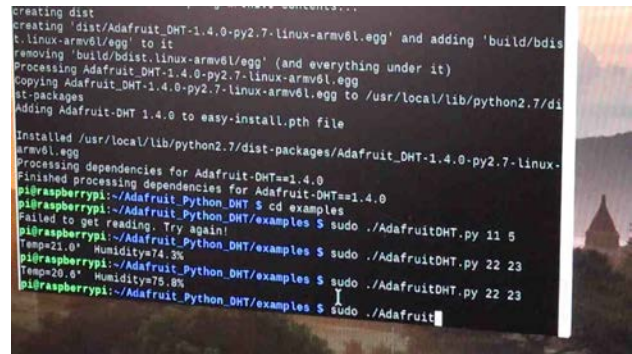
Figure 15. Appearance of the Raspbian shell showing the measurements of temperature and humidity from sensors
