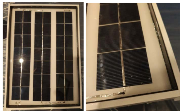
Figure 5. Mini battery, filled by epoxy resin
