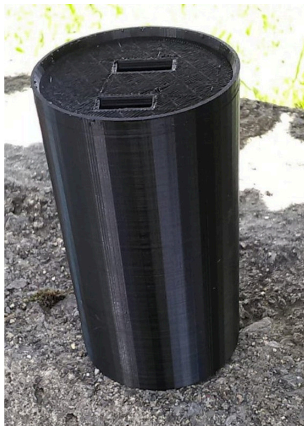
Figure 13. The external container made of black PLA
