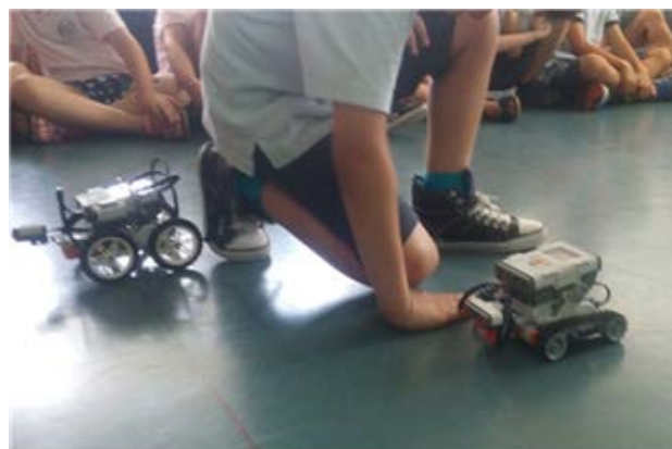
Figure 4. Using different sizes or types of “wheels” may demand adjusts to be done to the programming of the robot
