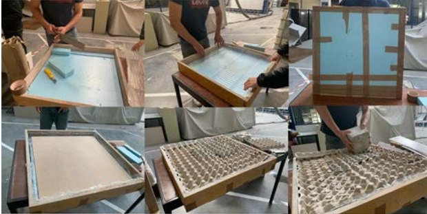
Figure 2. Model 2: styrofoam, wood, egg boxes, air bubbles plastic, plasterboard
