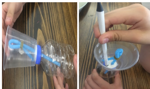
Figure 9. Joining the glass and bottle with adhesive paste
