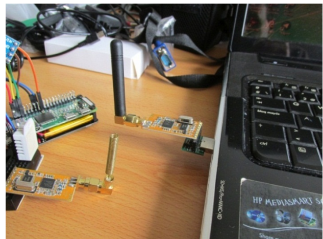
Figure 7. The pair of devices of the communication module: one attached to the computer and the on-board device
