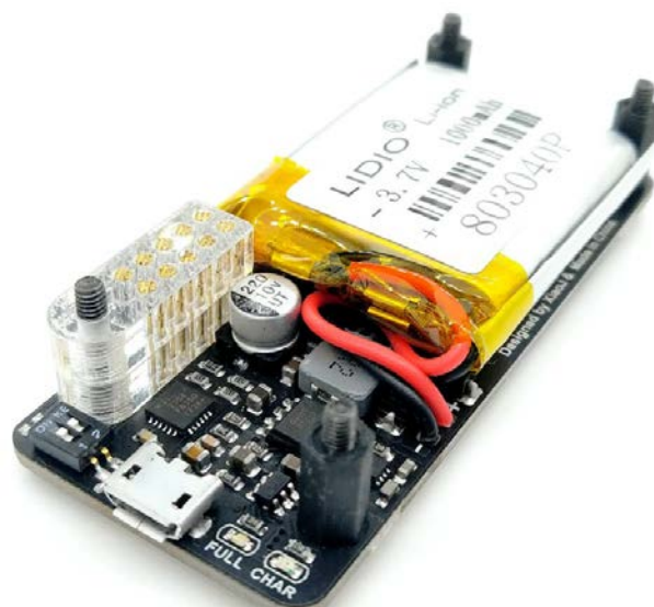
Figure 5. A lithium battery with regulation and measurement elements is used as a power supply
