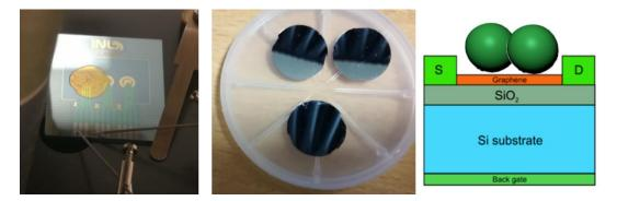
**Figure 3.7** Mass produced GFET, left. Microscope slide back gated, center. Schematic of the back gated transistor, right.
