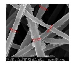
**Figure 4.6** SEM micrographs of the produced nanofibers. 3NA-PCL (left) and 2A4NA-PCL (right) hosted nanofibers.
