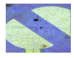
Figure 3.9 RRS spectra of CdSe QDs with a 5nm diameter (left). Active area of the liquid gate GFET, note the black area where the QDs agrgregated (right).
