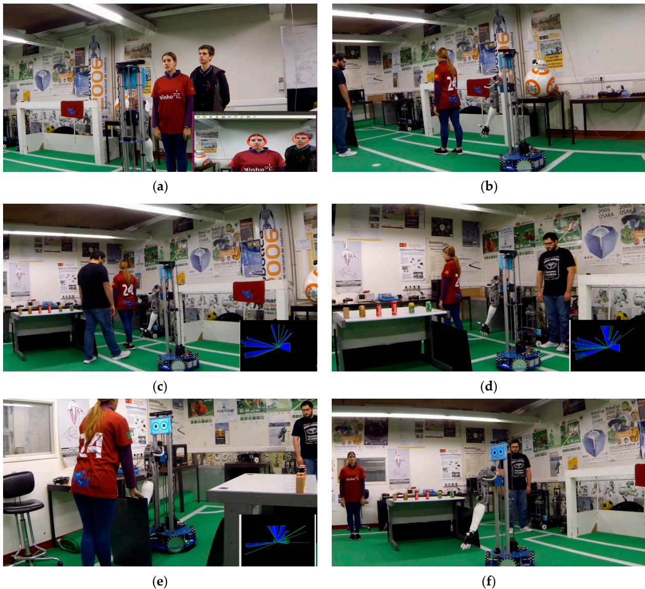
Figure 21. A step-by-step demonstration of CHARMIE’s “Follow Me” task. From receiving the task to navigating behind the human user while avoiding static and dynamic obstacles that cross the path between the robot and the user. When the robot cannot continue following the user, it recalculates a new trajectory.
