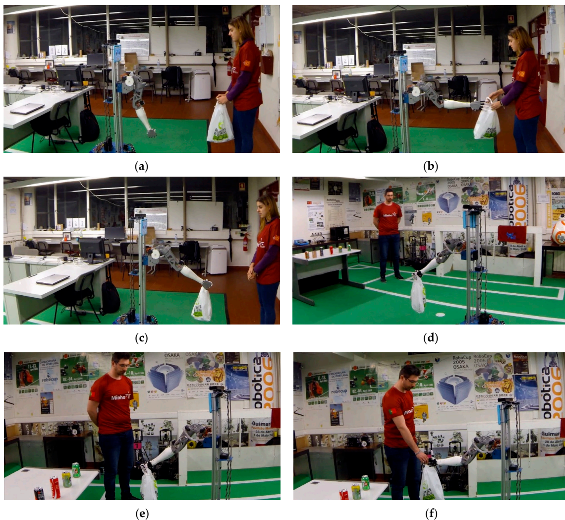
Figure 19. A step-by-step demonstration of CHARMIE's “Help me carry this bag” task. From receiving a task from the first user, collecting the bag, navigating to the desired location and hand-delivering it to the second user.
