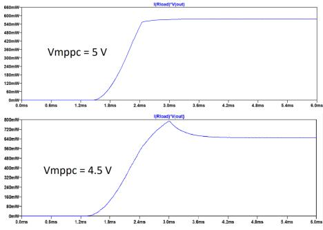
**Fig. 9.** Graphs of the output power of the converter when the PV module is not in ideal conditions (575 mW @ *V*<sub>MPPC</sub> = 5 V; 651 mW @ *V*<sub>MPPC</sub> = 4.5 V).
