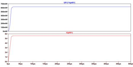
Fig. 6. Output power (624 mW) and voltage (5.58 V) in the equivalent circuit of the monocrystalline/polycrystalline module.
