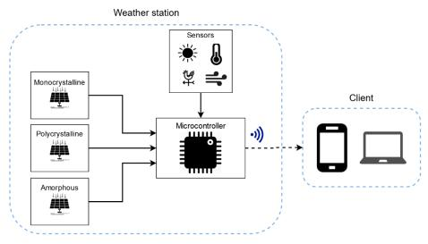
Fig. 1. System architecture in the context of a PV module evaluation system that integrates a weather station and a client machine (smartphone or computer).
