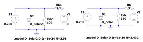
Fig. 3. Equivalent circuits and their components values for the photovoltaic modules: Amorphous module (left) and monocrystalline/polycrystalline modules (right).
