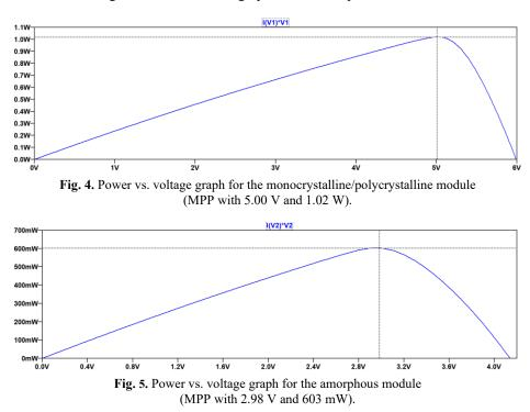
A 50  $\Omega$  load was added to the output of the equivalent circuit of the monocrystalline and polycrystalline module, in order to obtain the values of the output power without the converter, for comparison purposes. The graphs for both power and voltage of the
