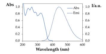
Figure 3. Normalized absorption and emission spectra of imidazole derivative 3.
