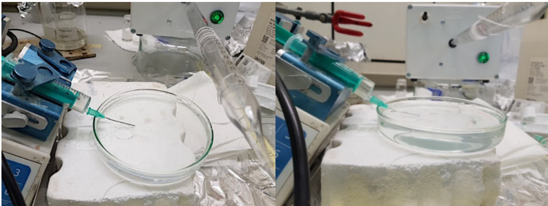
Figure 4.5 | Customized wet spinning setup for the continuous production of PCL/gelatin and PCL/gelatin/HAp microfibers.
