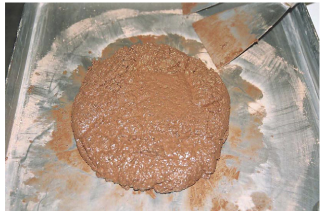
Fig. 2. Fresh TMWM mortar.
