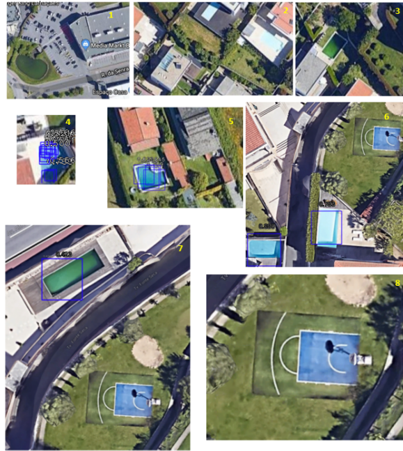
Fig. 5. Eight test images from Google Maps with different sizes and resolutions. The objects detected by RetinaNet+ResNet101 are surrounded by blue boxes. The images are numbered in the upper right corner.
