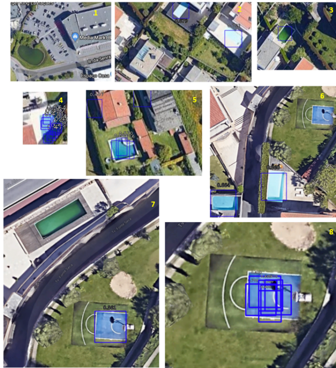
Fig. 4. Eight test images from Google Maps with different sizes and resolutions. The objects detected by RetinaNet+ResNet50 are surrounded by blue boxes. The images are numbered in the upper right corner.
