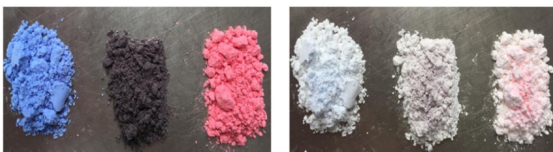
Figure 18: Thermochromic powders (blue, black and red) disactivated under 31 °C (left) and activated above 31 °C (right) [144]
