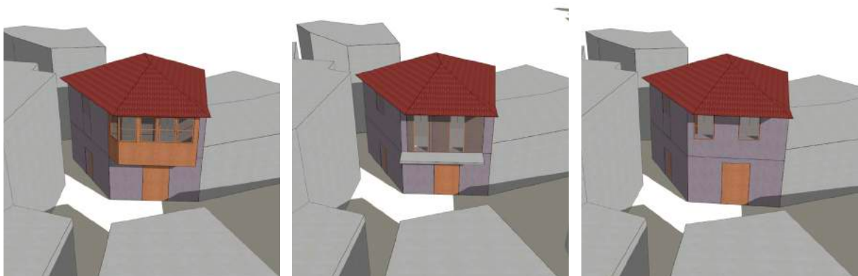
FIGURE 6.5. Case Study 2 – models of the three scenarios considered in simulations. (left) glazed balcony; (center) balcony; (right) no balcony, small windows.
