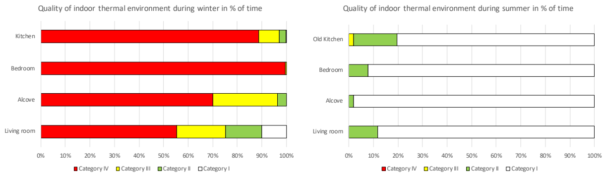
FIGURE 5.59. Classification of indoor thermal environment for representative rooms of the building. (left) Winter; (right) Summer.
