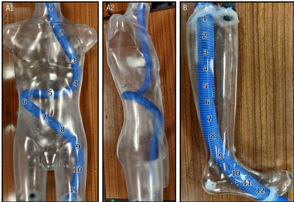
Figure 5.15 -Anatomical models of a human torso (A1 and A2) and lower leg (B) adapted to be filled with phantom, along with the pipe for the implant to travel in. The points where measurements were performed are marked in the photographs.
