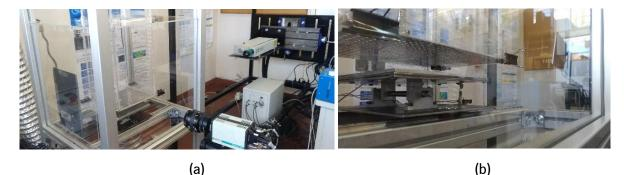
Figure 35. (a) PIV system; (b) measurement region.
