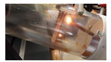
Figure 42. Auto-ignition of the olive oil particles inside the vaporizer.
