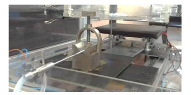
Figure 26. Apparatus to measure the total pressure at the setup exit.
