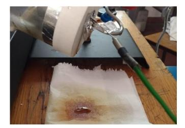
Figure 45. Partial evaporation of the olive oil particles at 10 V.
