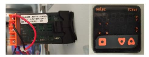
Figure 24. Temperature controller TC544A.
