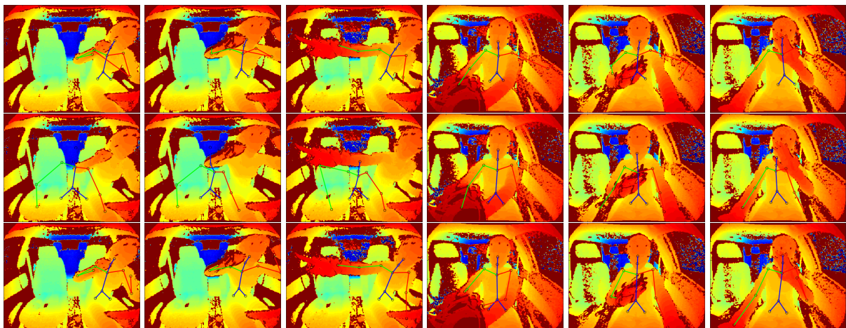
Figure 7.7: Joint failure quantitative results of the final human body pose detection method for three training configurations, FT# : (1 st row) represent FT1 in both ToF PoV scenarios; (2 nd row) represent FT2 in both ToF PoV scenarios; (3 rd row) represent FT3 in both ToF PoV scenarios; (1 st to 3 rd column) represent FM1 ; (4 th to 6 th column) represent FM2 . Joint failure is associated with proximity of the joint to the edge of the image (i.e. Wrists), or training error from ground-truth (i.e. proximity of the joint to the ToF sensor, or kinematic forwarding error propagation).
