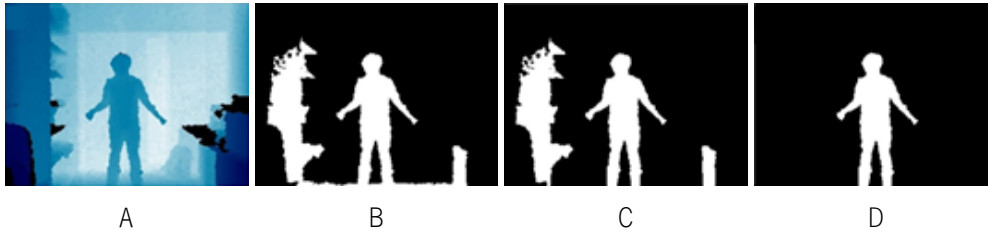
Figure 6.11: Human silhouette mask construction: (A) original image, (B) region growing result, (C) floor elimination, and (D) final mask.
