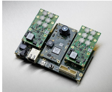
Figure 2.11: Melexis EVK75023 ToF sensor. Illustration adapted from [16].
