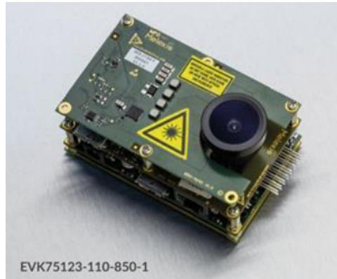
Figure 2.14: Melexis EVK75123 ToF sensor. Illustration adapted from [17].
