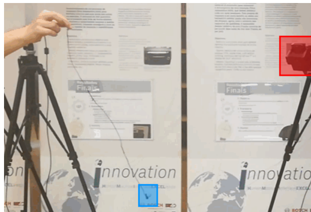
Figure 4.12: Marker pendulum motion capture through Vicon and ToF sensor, for temporal alignment between systems: blue highlight represents the Vicon marker, and red highlight represents the ToF camera.
