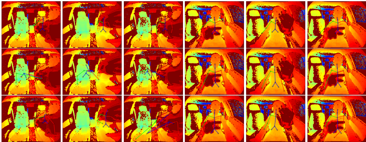
Figure 7.8: Full body failure quantitative results of the final human body pose detection method for three training configurations, FT# : (1 st row) represent FT1 in both ToF PoV scenarios; (2 nd row) represent FT2 in both ToF PoV scenarios; (3 rd row) represent FT3 3 in both ToF PoV scenarios; (1 st to 3 rd column) represent FM1 ; (4 th to 6 th column) represent FM2 . Full body failure is associated with missing feature information due to the presence of body parts in the ToF sensor dead-zone.
