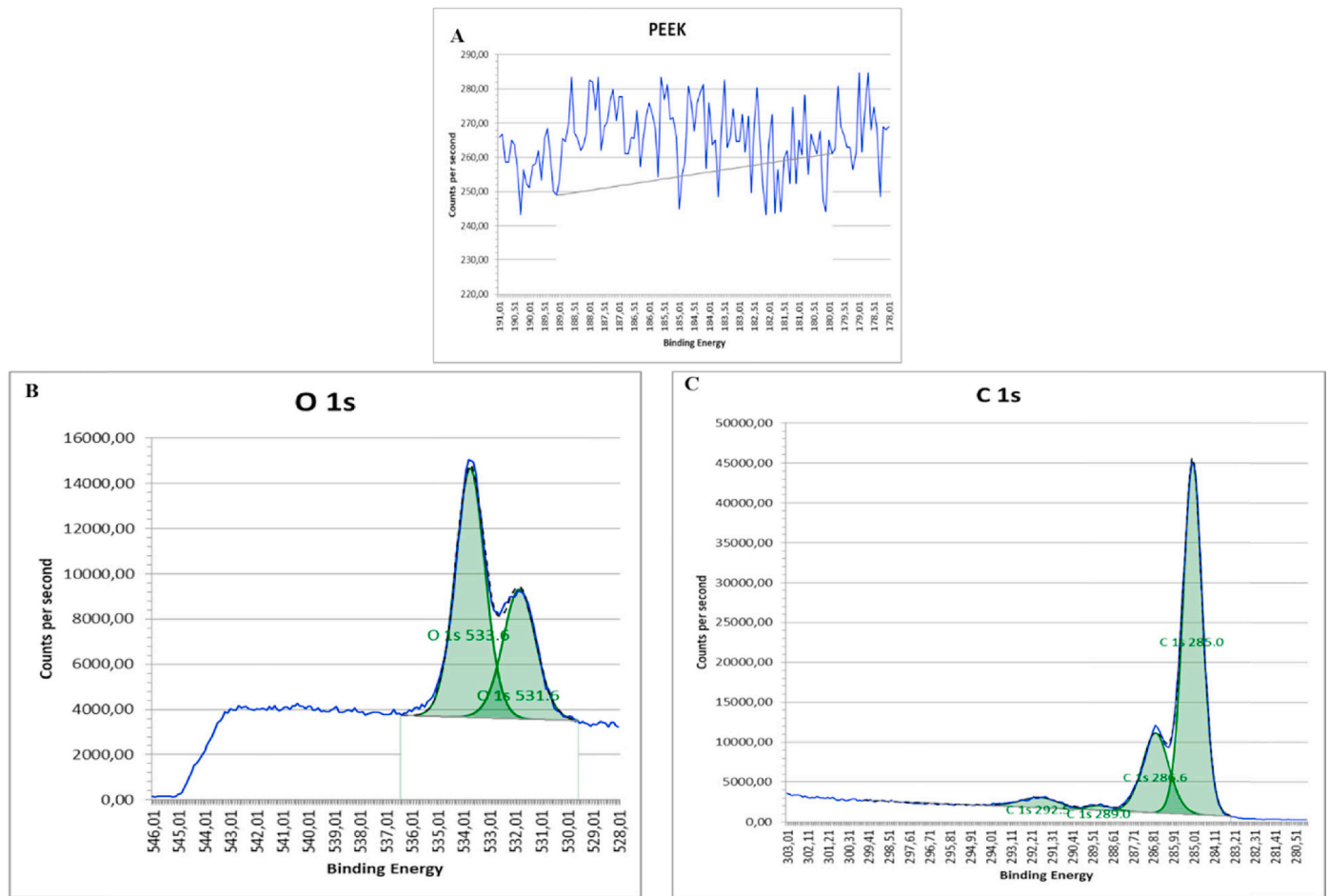
Fig. 4. XPS plot of PEEK. A) Survey scan XPS spectra showing O 1s and C 1s peaks; B) high-resolution XPS spectra of O 1s; and C) high-resolution XPS spectra of C 1s.
