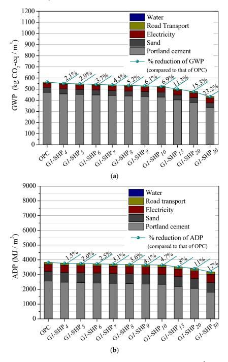
**Figure 3.** Comparison of (a) GWP and (b) ADP impacts of developing  $1 \text{ m}^3$  mortars using OPC with those of developed by G1-SH<sub>*i*</sub>.
