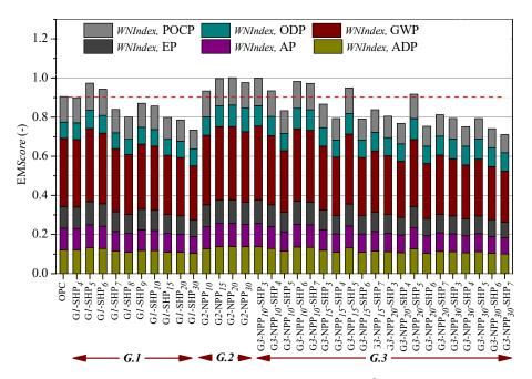
Figure 10. Comparison of the EMScore calculated for 1 m<sup>3</sup> of the mortars made of the developed cements.
