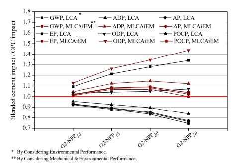
**Figure 8.** Ratio of GWP and ADP impacts produced by development of  $1 \text{ m}^3$  mortar using G2-NPP<sub>i</sub> cements to that of produced by  $1 \text{ m}^3$  mortar made of OPC.
