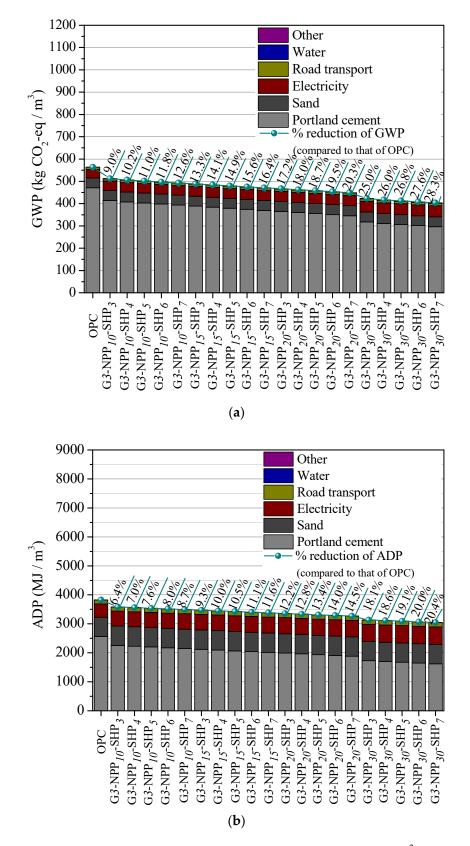
**Figure 5.** Comparison of (**a**) GWP and (**b**) ADP impacts of developing 1 m<sup>3</sup> mortars using OPC with those of developed by G3-NPP<sub>*i*</sub>-SHP<sub>*i*</sub>.
