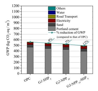
Figure 6. Comparison of GWP impact of developing 1 m<sup>3</sup> mortars using different cements.
