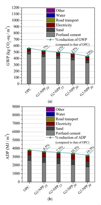
**Figure 4.** Comparison of (a) GWP and (b) ADP impacts of developing  $1 \text{ m}^3$  mortars using OPC with those of developed by G2-NPP<sub>*i*</sub>.
