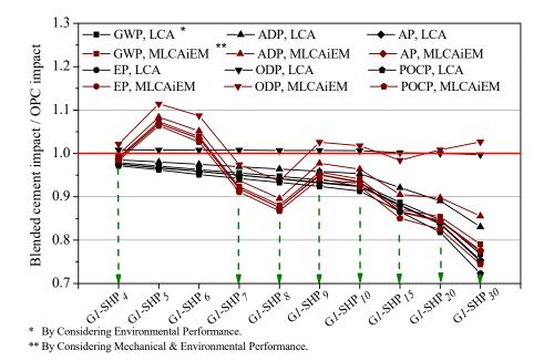
**Figure 7.** Ratio of GWP and ADP impacts produced by development of  $1 \text{ m}^3$  mortar using G1-SHP<sub>*i*</sub> cements to that of produced by  $1 \text{ m}^3$  mortar made of OPC.
