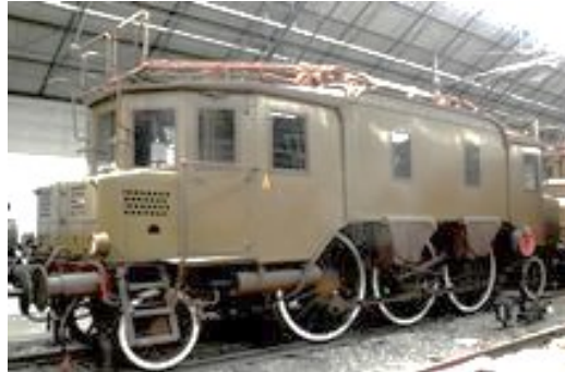
Figure 2.1. E330 three-phase Italian locomotive in the period 1914–1963 [69]. Source: [ https://books.google.com/books/about/Italian_Railways.html?id=JFcSAAAAMAAJ ].
