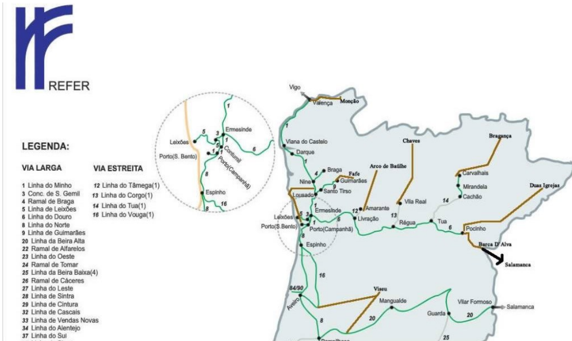
Figure 1.5. Railway network in north of Portugal plus the already abandoned rail lines (in brown) [15]. Source: [Infraestruturas de Portugal].
