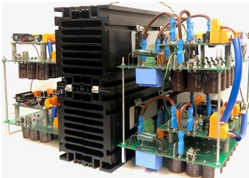
Figure 5.32. Single MMC leg/phase (four SMs).
