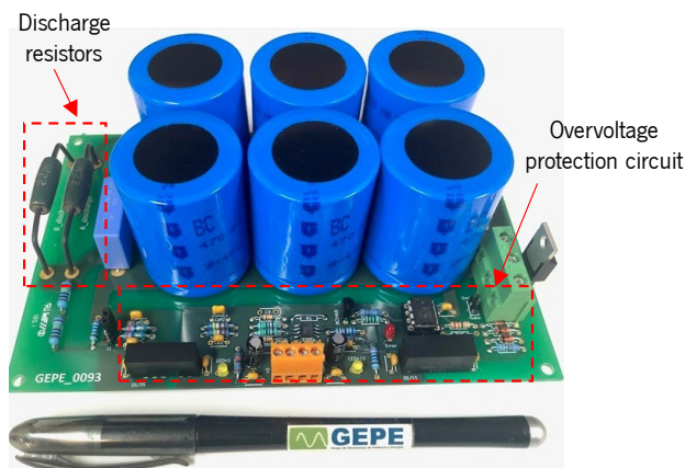
Figure 5.35. Main DC-link capacitor (developed under the scope of this Ph.D. thesis).
