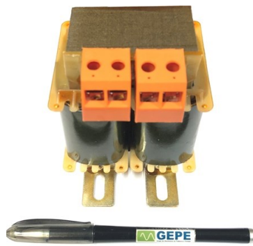
Figure 5.33. Filter inductor used in MMC.
