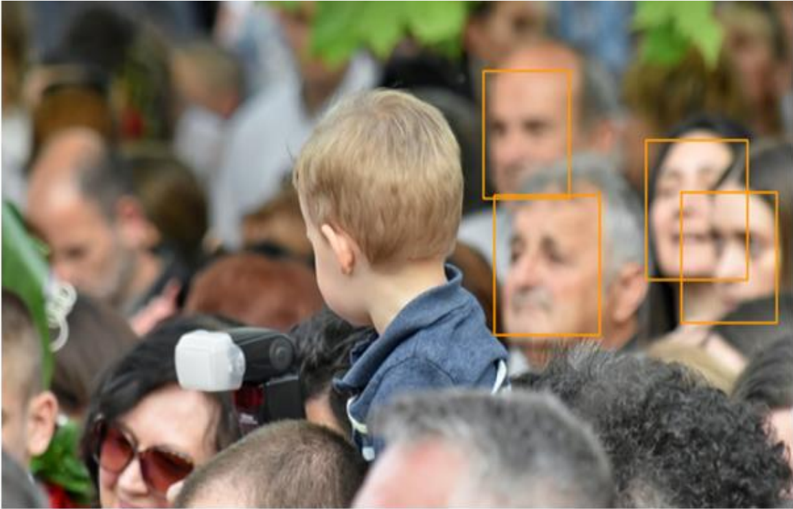
Figure 62 - Bounding box output on images containing blurred faces. Photo covered by Creative Commons license
