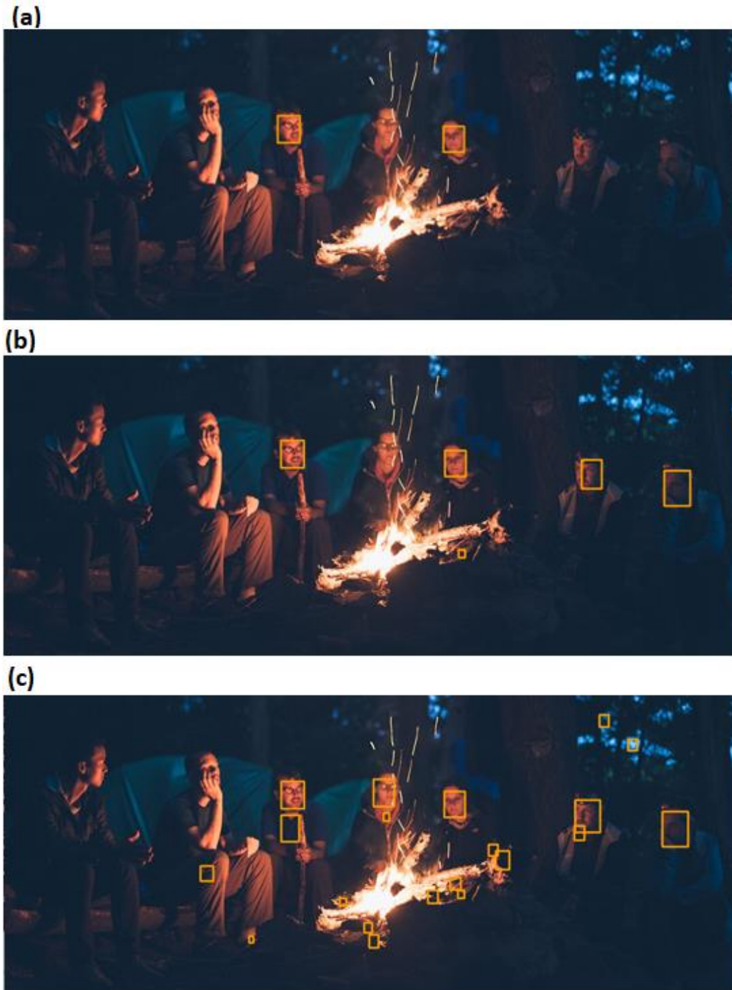
Figure 64 - MTCNN bounding box output on comparison on a low illumination background with different threshold arrays (2). (a) - [0.6, 0.7; 0.7]; (b) - [0.5, 0.6; 0.6]; (c) - [0.4, 0.5; 0.5]. Photo under Creative Commons License
