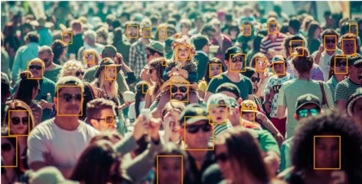
Figure 65 – MTCNN output on harder faces to characterize with different threshold arrays. (a) - [0.6, 0.7; 0.7]; (b) - [0.5, 0.6; 0.6]. Photo covered by Creative Commons license
