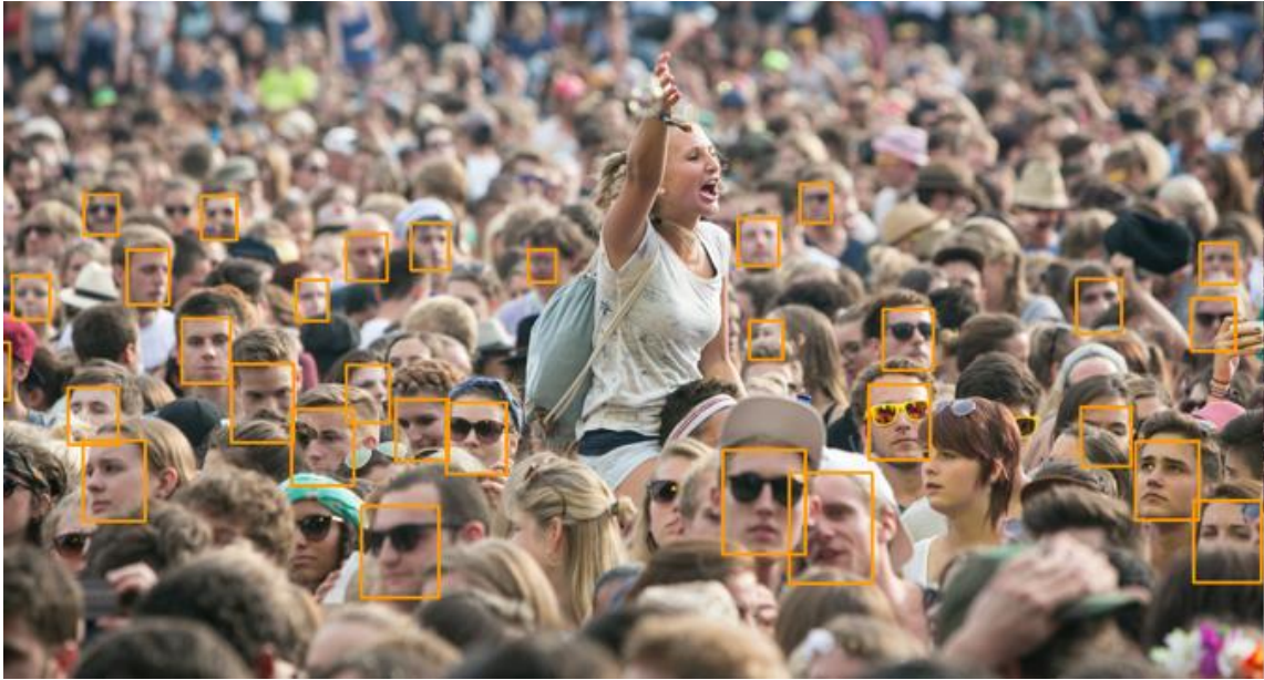
Figure 60 - MTCNN bounding box output Mob image showcasing different detected face pose variations with [0.6,0.7,0,7] threshold array. Photo by Michael Dornbierer covered by Creative Commons license
