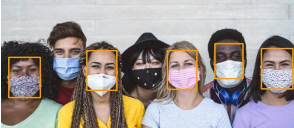
Figure 66 - MTCNN bounding box results on an image of people wearing masks. Royalty Free photo taken online
