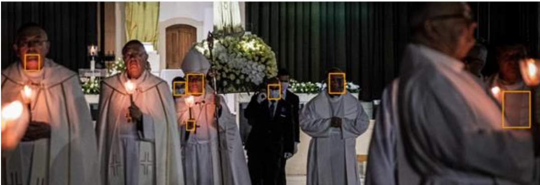
Figure 63 -MTCNN bounding box output comparison on a low illumination background with different threshold arrays (1). (a) - [0.6, 0.7; 0.7]; (b) - [0.5, 0.6; 0.6]; (c) - [0.4, 0.5; 0.5]
