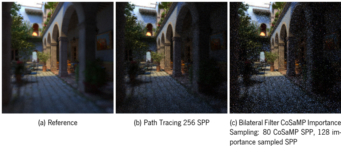
Figure 8.16: Image Comparison of the Bilateral Filtered Importance Map approach to Path tracing for the San Miguel scene
