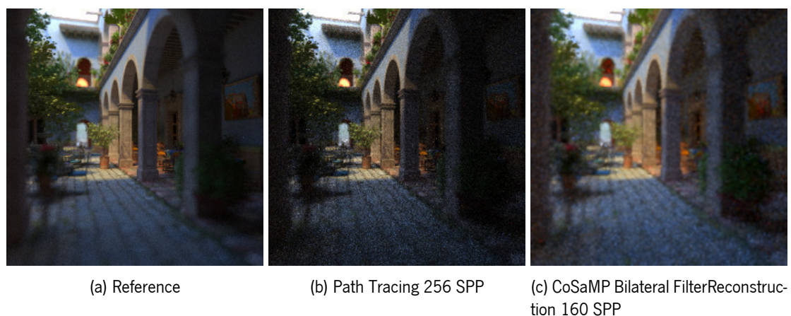
Figure 8.9: Image Comparison of the CoSaMP approach to Path tracing for the San Miguel scene
