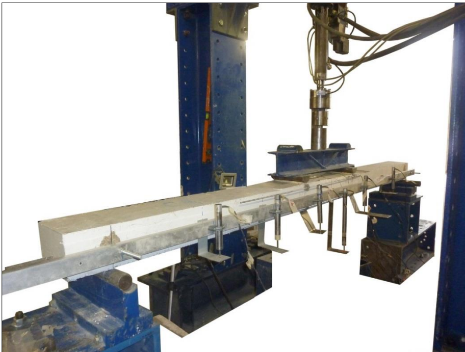
Figure 3.19: View of four-point bending test
