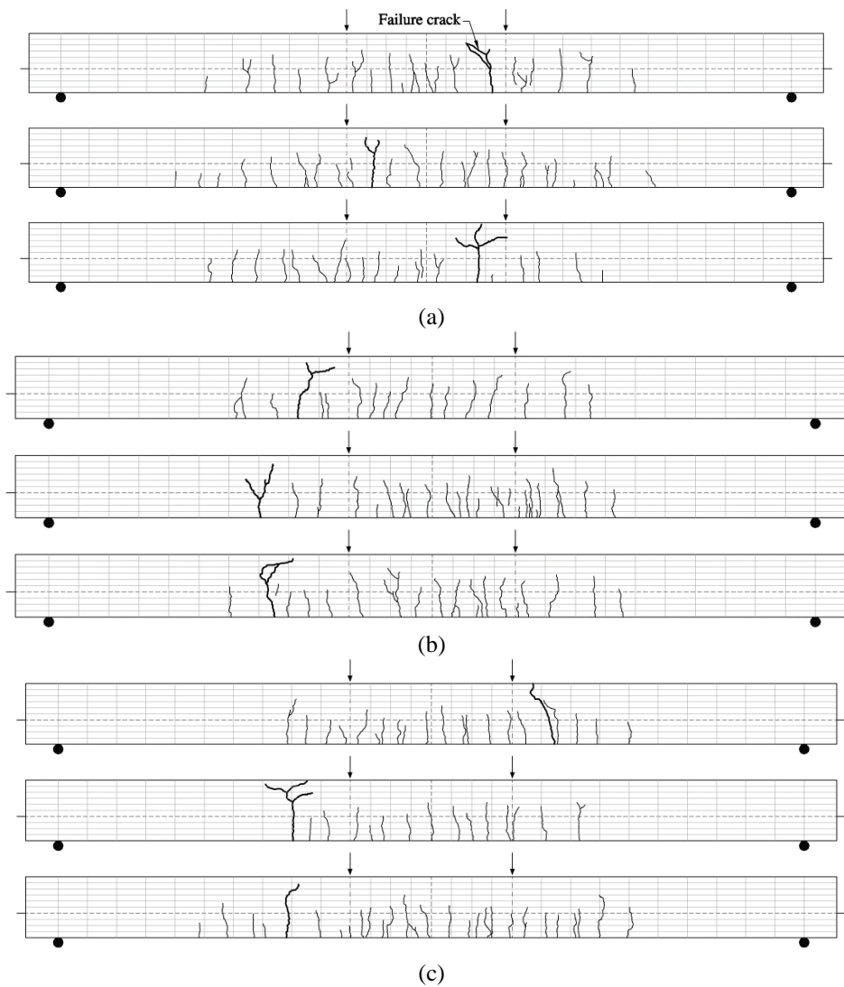
Figure 3.24: Ultimate crack pattern of (a) SR/FRC1545, (b) SR/FRC2560, and (c) SR/FRC4590 series beam
