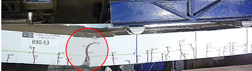
Figure 3.23: Crack failure localisation in SR/FRC beam
