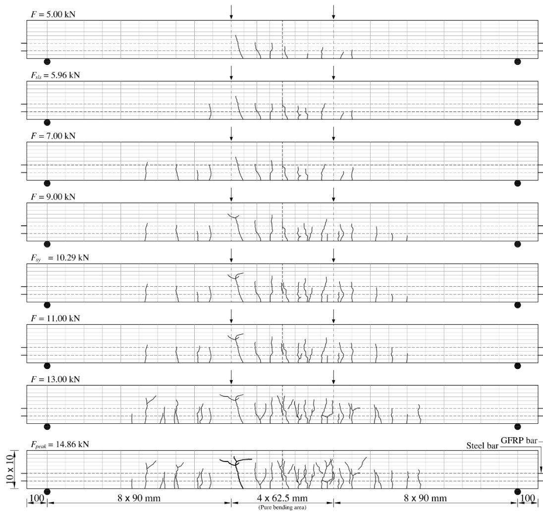
Figure B.9: Crack evolution in SGR/FRC4590-3
