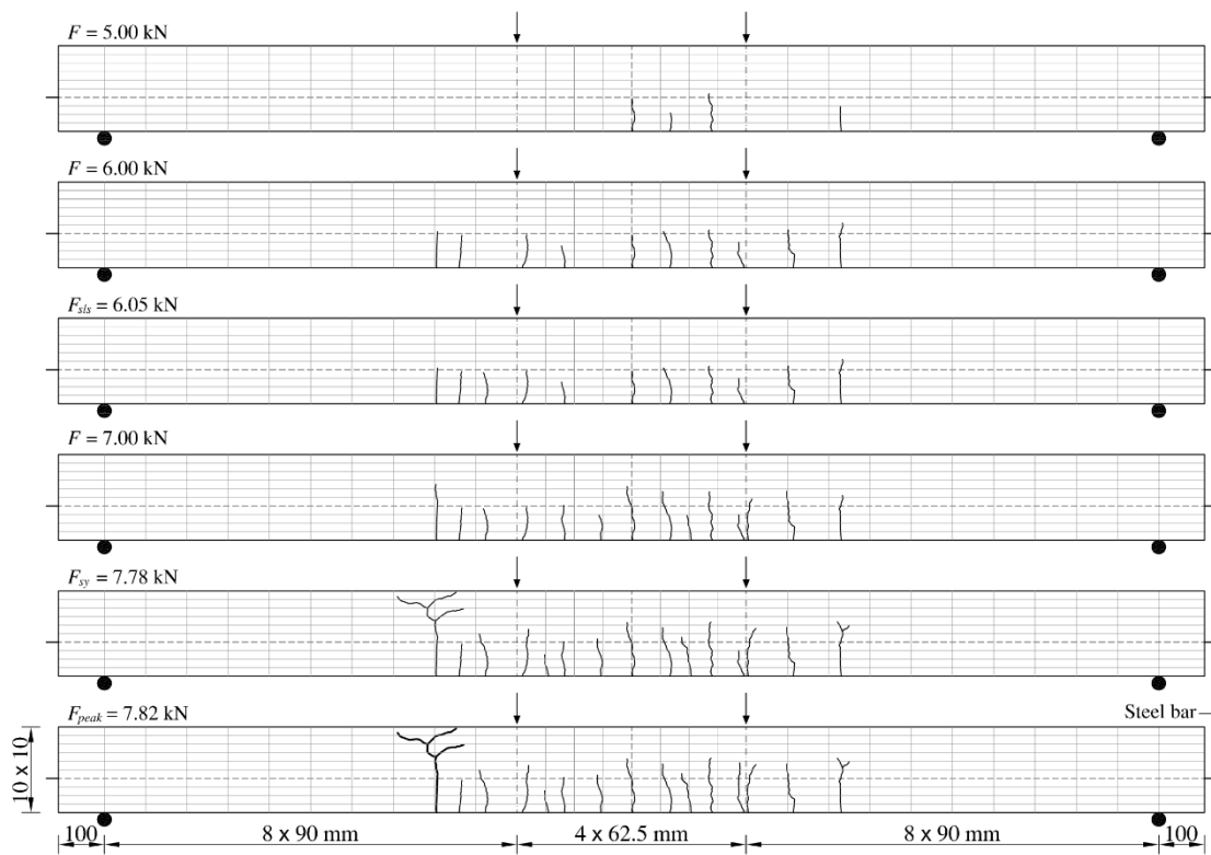
Figure A.8: Crack evolution in SR/FRC4590-2
