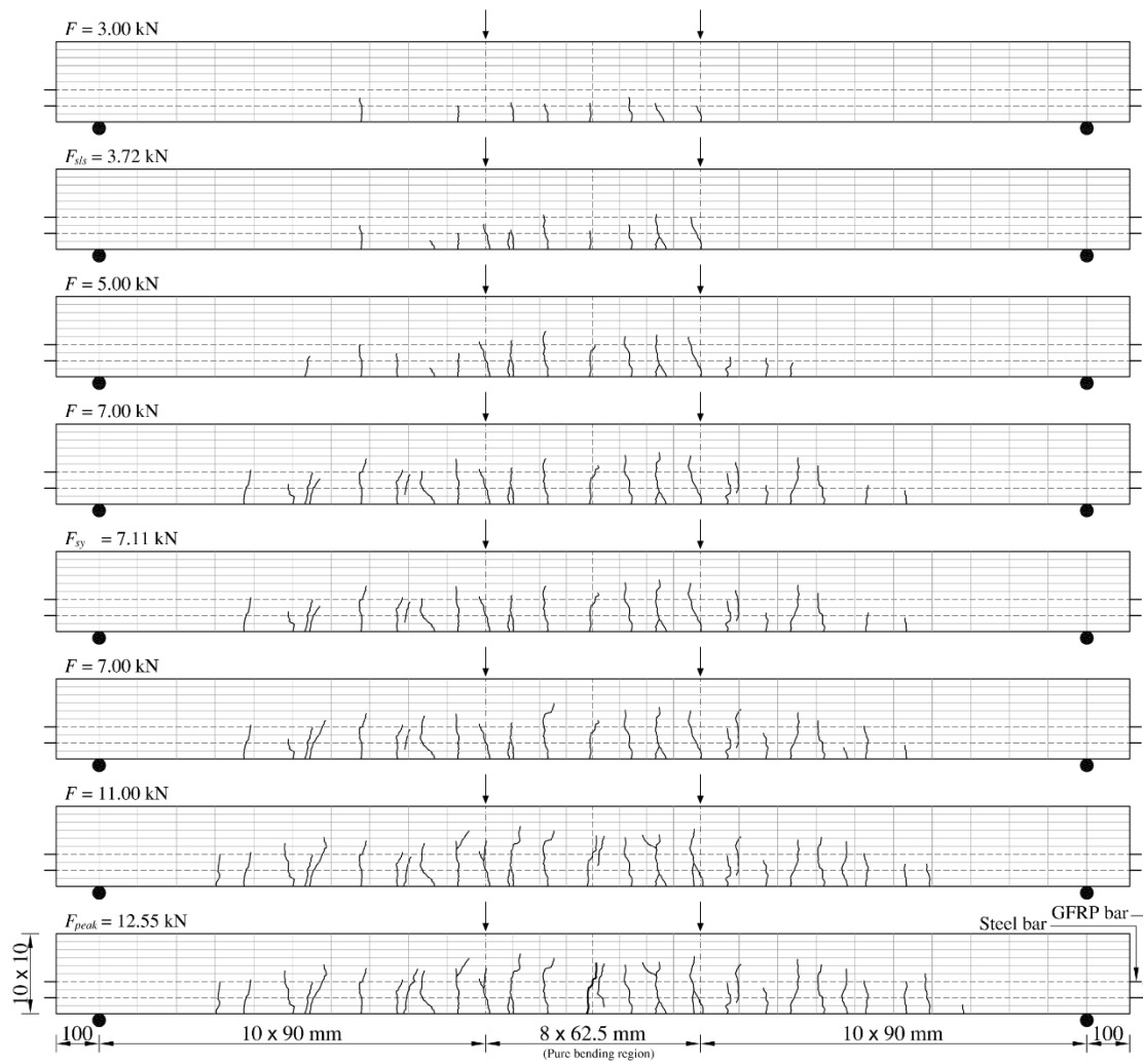
Figure B.3: Crack evolution in SGR/FRC1545-3
