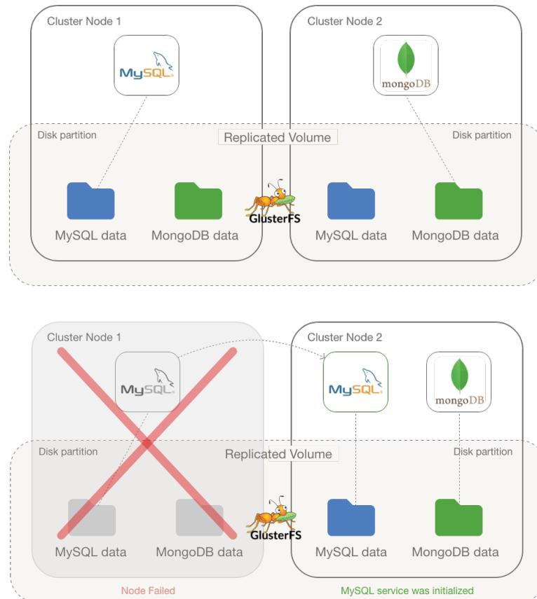
Figure 31: Failure of a statefull service
