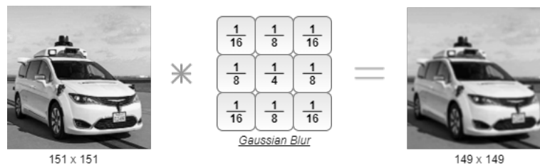
Figure 5.13: Voting convolution with a Gaussian Blur filter
