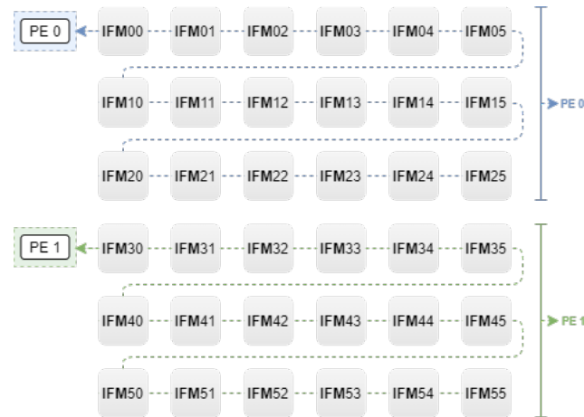
Figure 3.10: Convolution parallelism with stride 3
