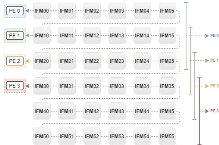
Figure 3.9: BSM architecture parallelism
