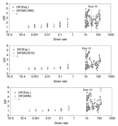
Figure 5. Comparison of experimental DIF with DIF obtained from MC 1990, MC 2010 and proposed ANN model.
