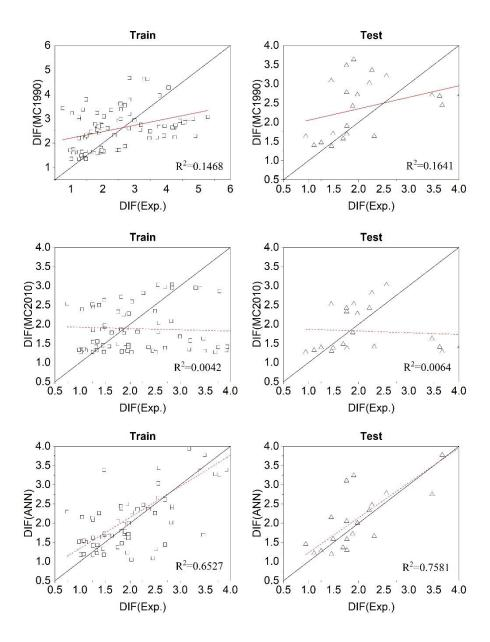
Figure 4. Comparison of DIF obtained from MC 1990 and MC 2010 models and ANN with corresponding experimental values strain rates higher than intermediate level.
