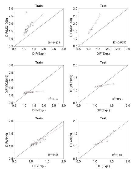
Figure 3. Comparison of DIFs obtained from MC1990 and MC2010 and ANN-model with corresponding experimental values for strain rates lower than intermediate level
