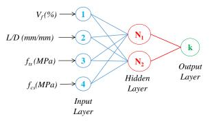
Figure 1. Architecture of the comprehensive version of the proposed network.
