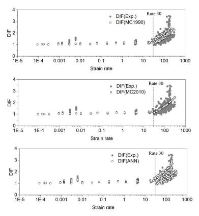
Figure 2. Comparison of experimental DIF with DIF obtained from MC 1990, MC 2010 and proposed ANN model (Ramezansefat et al. 2020).
