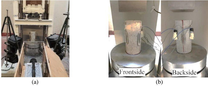
Figure 2. (a) The drop weight impact machine and (b) Cylinders under impact test.
