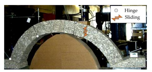
Figure 4. Deformed shape of the arch at the ultimate displacement, retrieved from [35].
