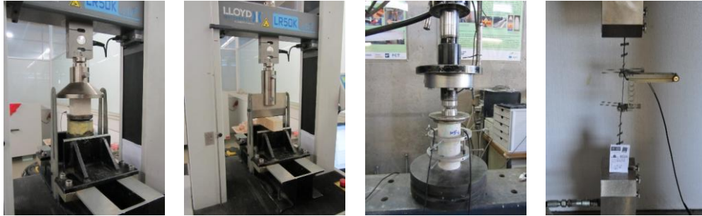
576 Fig. 2. Material characterization tests: (a) compressive test; (b) flexural test; (c) elastic modulus 577 test; (d) fabric direct tensile test. 578
