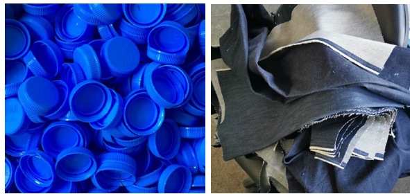
Figure 1. Matrix and reinforcement materials
