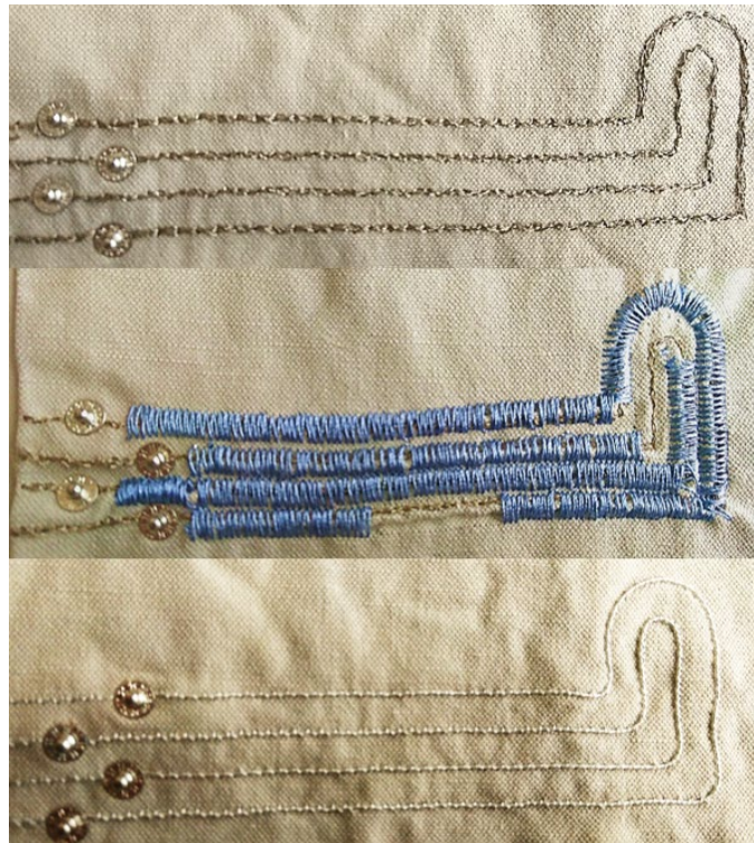
Figure 1: Types of conductive tracks used in detergent evaluation. Top: direct embroidery (DIR), middle: direct embroidery with non-conductive overlay (OVR), bottom: TFP embroidered sample (TFP).
