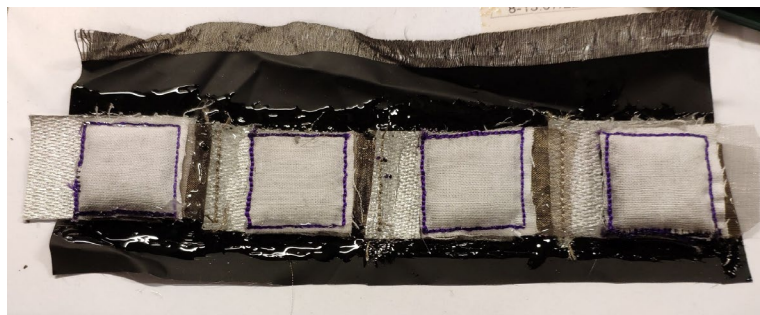
Fig. 5. Inner structure of a multi-cell battery with sealant applied
