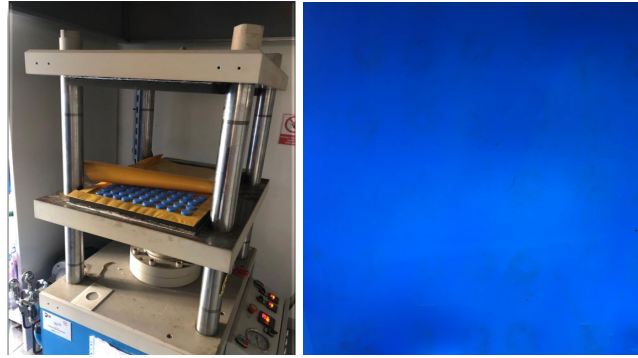
Figure 3. Hot press machine and the produced matrix plate
