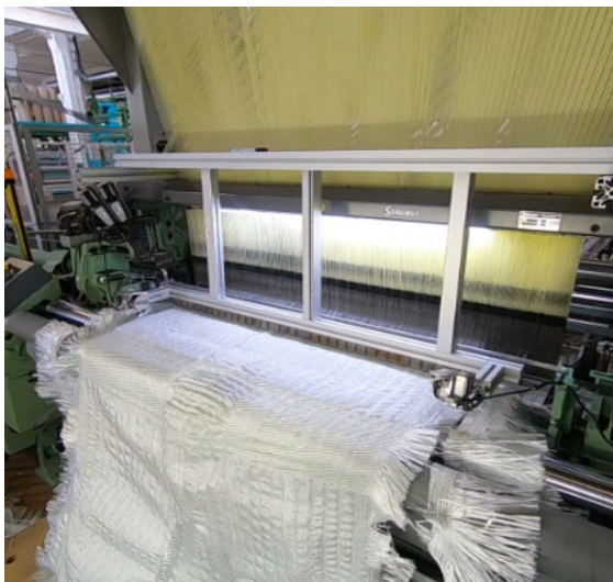
Figure 4: Installation of the weft yarn retention system
