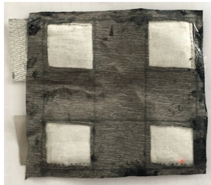
Fig. 4. Prototype of a multi-cell flexible textile Al-Air battery with 2x2 cell arrangement
