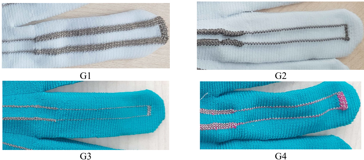
Fig. 3 Different knitted sensor designs Intarsia (G1), Intarsia (different layout; G2), plated with elastane (G3), plated with base material (G4)
