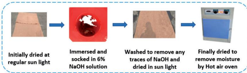
**Figure 2.** Alkali treatment process of jute fabric. J: jute fabric; G: E-glass fabric; GP: graphite particulate.
