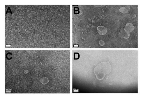
Fig. 6. TEM images of liposome-SF hydrogels (A) A1-SF, (B) B1-SF, (C) C1-SF and (D) D1-SF (scale bar = 100 nm). The liposomes were mixed with SF solution before coating on TEM grids and stained. The acceleration voltage of 200 kV was applied.
