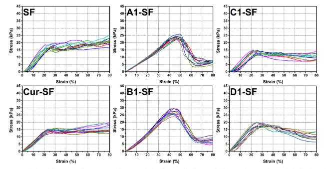
Fig. 7. Stress–strain plots of the regenerated SF, Cur-SF, and liposome-SF hydrogels assessed by the unconfined compression tests. The samples in disc shape with 5mm diameter and 2-mm thickness were immersed in PBS buffer for 24 h prior to mechanical analysis. Each line represents the data obtained from each tested sample.
