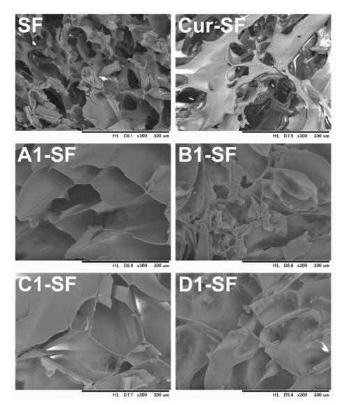
Fig. 5. SEM images freeze-dried SF, Cur-SF, and liposome (A1, B1, C1, D1)-SF hydrogels. Scale bar of SEM images is 300 µm.
