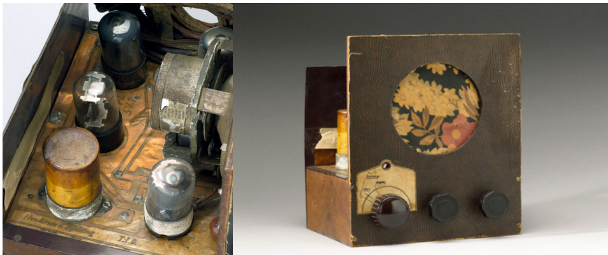
Figure I-9- Radio with printed PCB, in 1943 [73].
