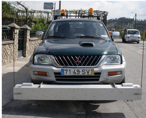
Figure 8. University of Minho and Coimbra High Speed Profilometer
