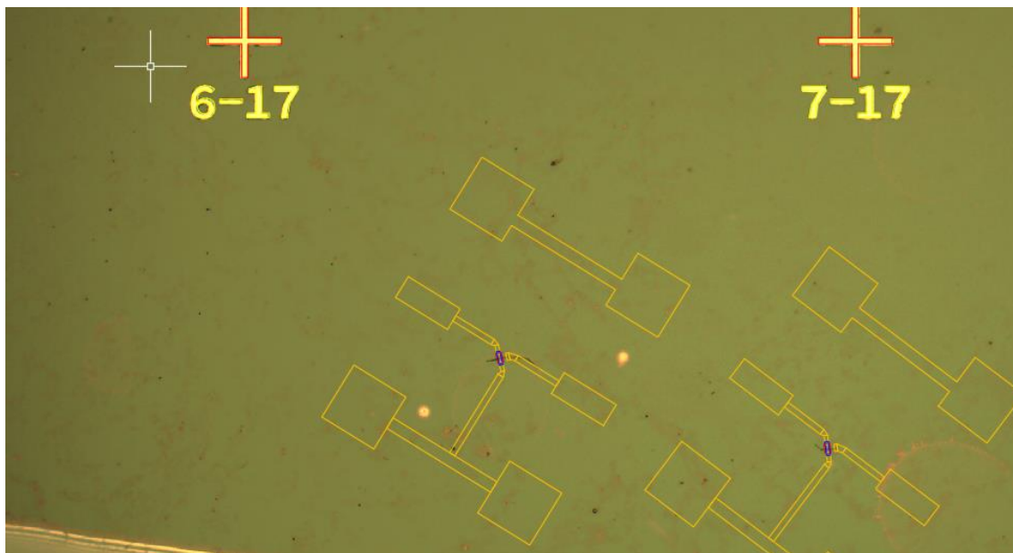
Figure 53: AutoCAD drawings with the overlaid image of the substrate containing the nanowires.
