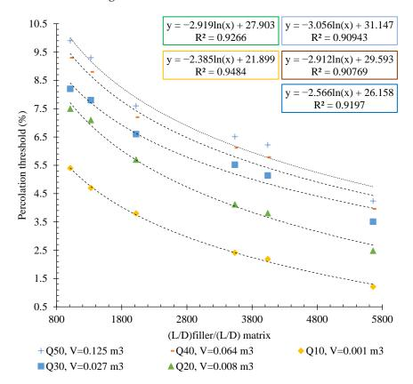
**Figure 14.** The relative aspect ratio of the carbon-based fillers vs. percolation threshold for the specimens with different volumes.
