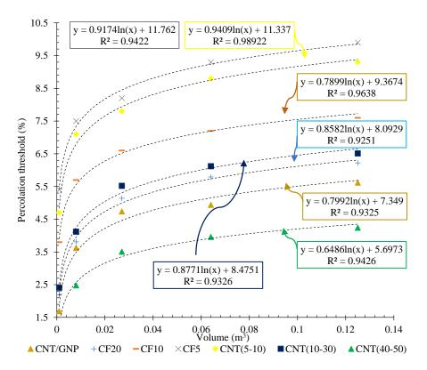
**Figure 15.** The percolation threshold vs. matrix volume (surrounded between electrodes) for the different CF and CNT reinforced specimens.
