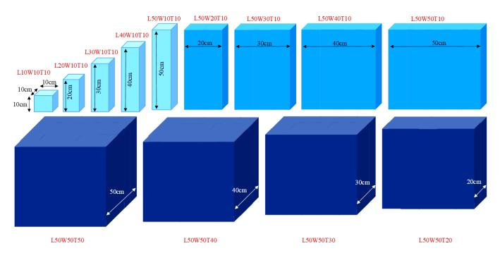
**Figure 2.** Schematic diagram of the specimens' dimensions (reinforced by hybrid CNT/GNP, 1:1), L: length, W: width, T: thickness.
