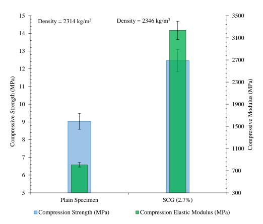
**Figure 19.** Mechanical properties of the 15 cm cubic specimen reinforced with 2.4% of CNT/GNP (SCG 2.7%).
