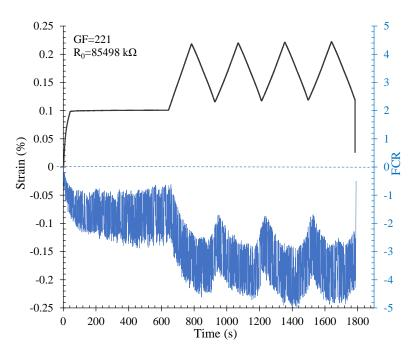
Figure 17. Piezoresistivity response of the cubic specimen under compression cyclic loading.
