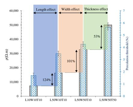
**Figure 12.** Electrical resistivity of specimens reinforced with hybrid CNT/GNP at the percolation threshold content.
