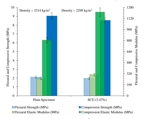
**Figure 18.** Mechanical properties of the  $10 \times 10 \times 85$  cm<sup>3</sup> beam reinforced with 3.47% of CNT/GNP (SCG 3.47%).
