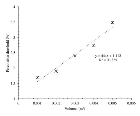
**Figure 9.** Relation between electrical percolation threshold and matrix volume of CNT/GNP reinforced specimens with different lengths.
