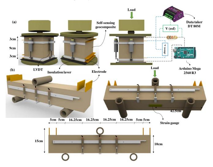
Figure 5. Test setup and electrode configuration: (a) compression, (b) flexural.
