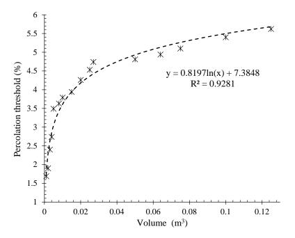
**Figure 13.** Relation between electrical percolation threshold and matrix volume for CNT/GNP reinforced specimens with different volumes.
