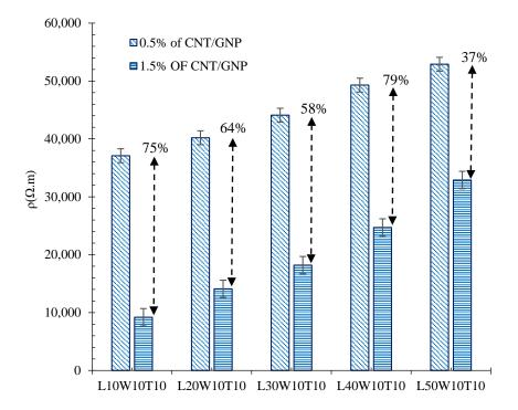
**Figure 8.** Volumetric electrical resistance of the specimens with different lengths and reinforced by 0.5 and 1.5% CNT/GNP.
