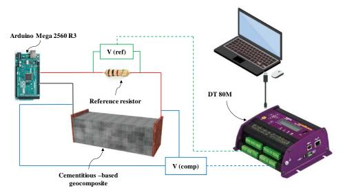
Figure 4. Experimental test configuration for electrical resistance measurement.
