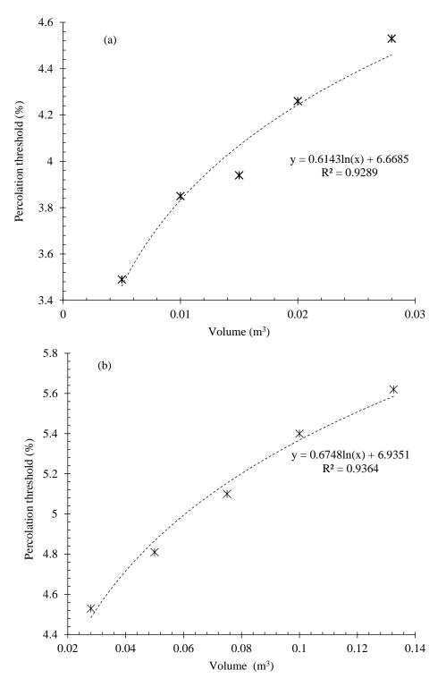
**Figure 11.** Relation between electrical percolation threshold and matrix volume for CNT/GNP reinforced specimens with: (**a**) different width, (**b**) different thickness.
