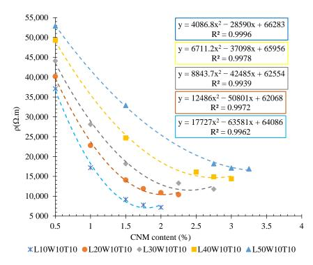
**Figure 7.** Volumetric electrical resistance of CNT/GNP-reinforced specimens with different lengths (surrounded between electrodes).
