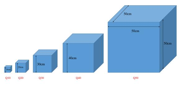
increased, as shown in Figure 3. The reason for choosing cubic specimens was to ignore the effect of changes in the aspect ratio of the matrix.
