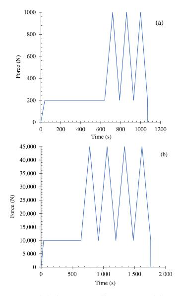
**Figure 6.** Cyclic loading patterns used for piezoresistivity behaviour investigations: (**a**) flexural mode, (**b**) compression mode.
