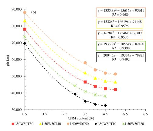
**Figure 10.** Volumetric electrical resistance of CNT/GNP reinforced specimens with: (**a**) different width, (**b**) different thickness.
