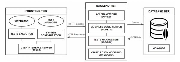
Figure 6. Architecture for self-diagnosis test system.
