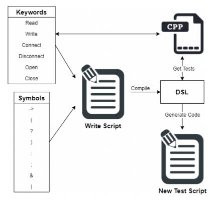
Figure 5. Proposed architecture for KDT with DSL.
