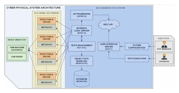
Figure 7. Architecture for a self-diagnosis test system integrated with the CPS.
