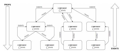
Figure 8. Interactions between components.
