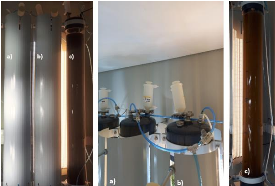
Figure 25: Bubble column photobioreactors, a) with a back and front metal sheet yellow light system, b) with a back and front metal sheet white light system, and c) with a front metal sheet yellow light system.
