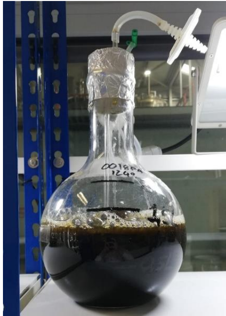
Figure 9: 1.5 L balloon reactor.
