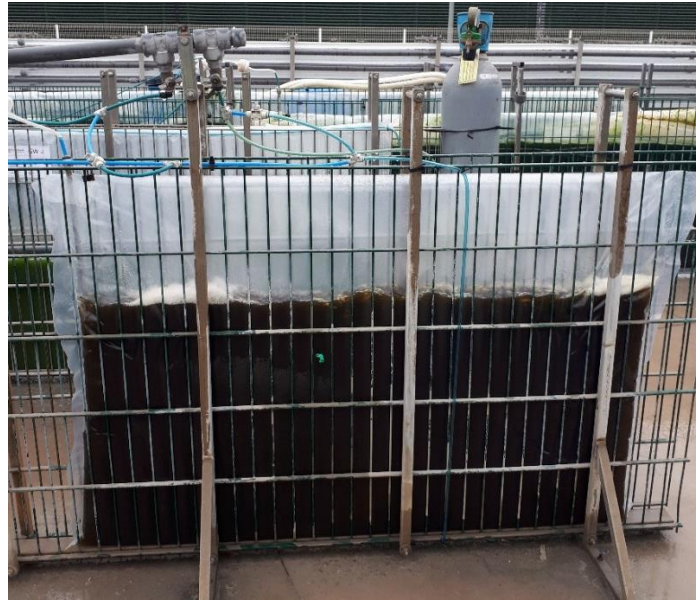
Figure 10: 70 L flat panel photobioreactor.
