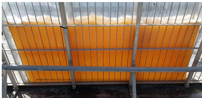
Figure 20: Phaeodactylum tricornutum cultivated in 70 L flat panels photobioreactor presenting a yellow color, which indicated death.
