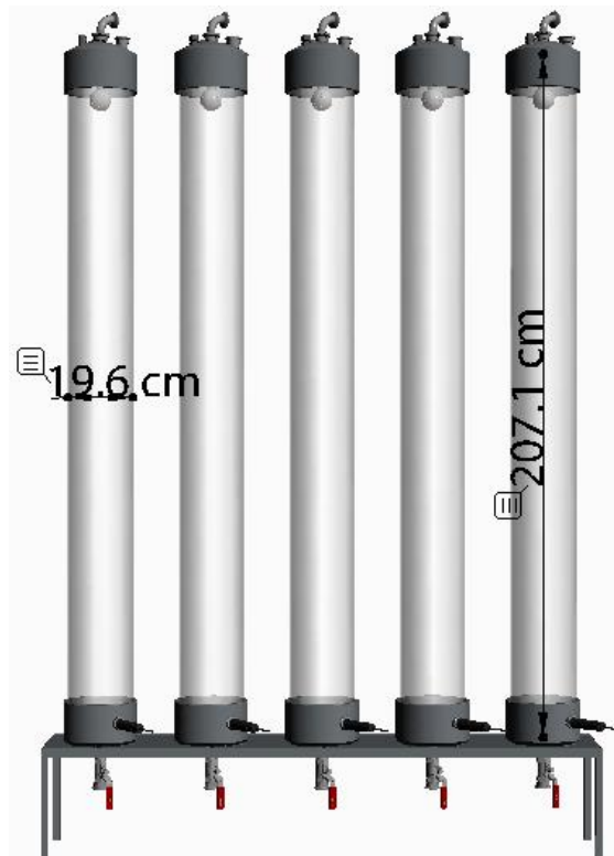
Figure 14: Bubble column photobioreactor system 3D design, with height and width measurements (Allmicroalgae designs).
