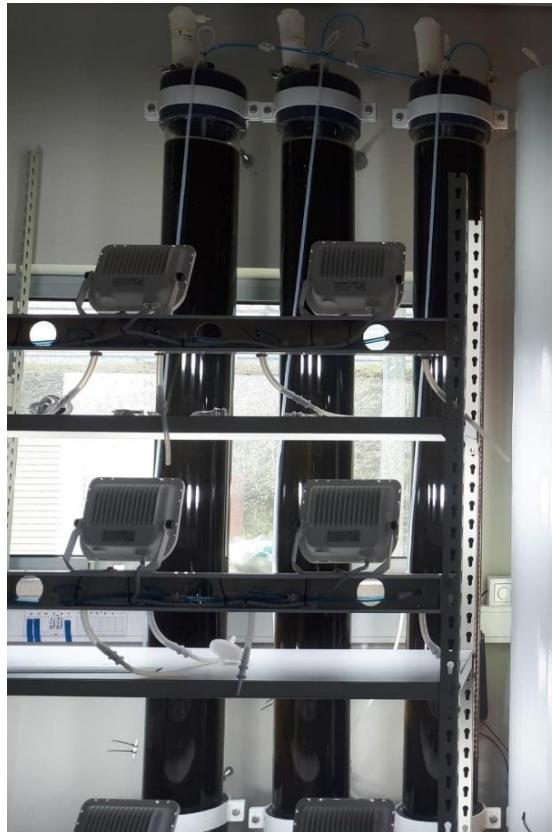
Figure 17: Three 60 L bubble column photobioreactors and the light column used.
