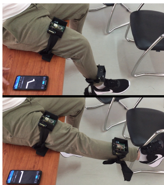
Figure 14. Wearable system and mobile app recognizing the movement of a volunteer's leg.
