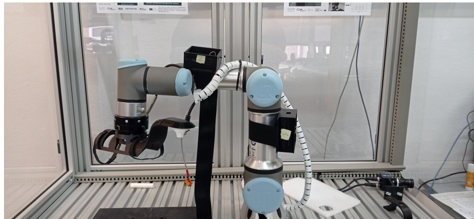
Figure 8. Wearable modules attached to the UR3 robot.
