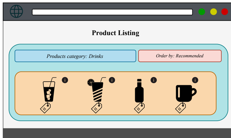
Figure 4.13: Product listing page recommendations vitrine generic template. In this example, the user browses for products within the "Drinks" category and orders them with the "Recommended" option. Ergo, products related to "Drinks" are listed, ordered by recommendation score, i.e., the products that would appeal the most according to the user's profile are shown first.
