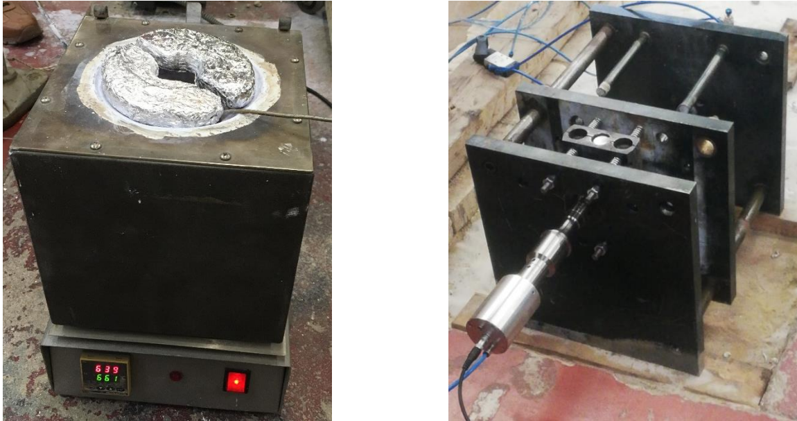
Figure 3.2 - Experimental apparatus: (a) Resistance melt furnace equipped with a SiALON Crucible; (b) Mold-Ultrasonic system assembly.
