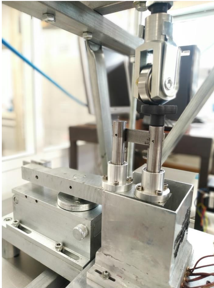
Figure 5.7 Test rig developed for the piston ring tribological assessment.
