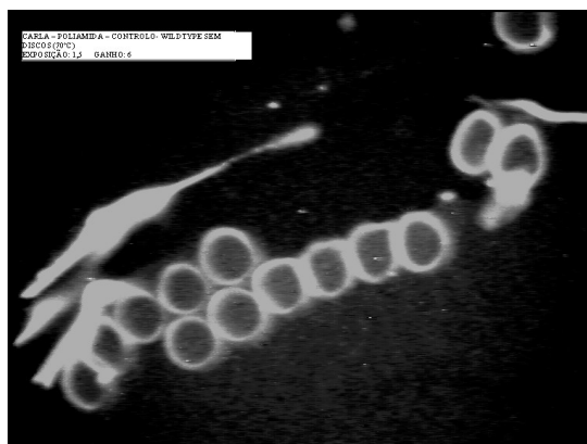
Figure 5.1 - Microscopic image of the polyamide stained samples (the reactive dye is linked only at the surface of the fibre).
