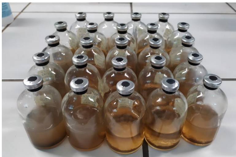
Figure 18: Aerobic assay vials, with PE, PET, PCL, and cellulose in film and powder, and the three blank assays.
