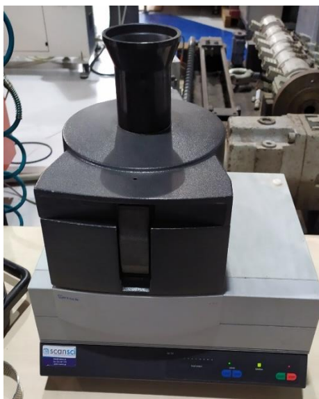
Figure 16: Mechanical grinder used to form the polymer powders used in the experiments.
