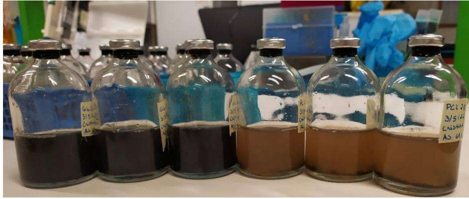
Figure A3.8: Aerobic assays triplicates with powder: with cellulose (on the left) and with PCL (on the right). Visible darkening of the growth medium.
