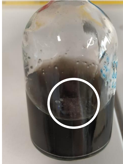
Figure A3.4: PE film observed floating at the surface of the anaerobic growth medium
