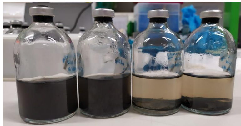
Figure A3.5: Anaerobic assays with PE (on the left) and PET (on the right) films duplicates
