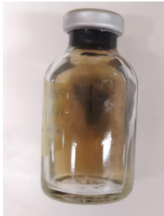
Figure 13: Vials used in the first biodegradation experiment. The darker powder on the walls of the vials is the leachate biomass.
