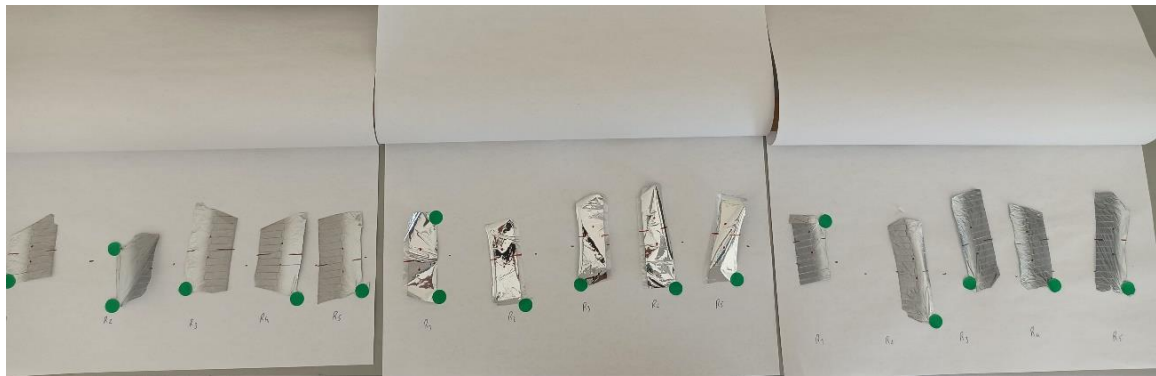
Figure 23 - Sample's specimens used to study the shrinkage behaviour.
