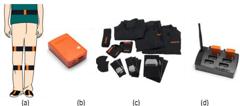
Figure 3-3 – Xsens MVN Awinda components. (a) lower body configuration; (b) MVN Motion Tracker (MTw); (c) MVN Awinda straps; (d) MVN Awinda station.
