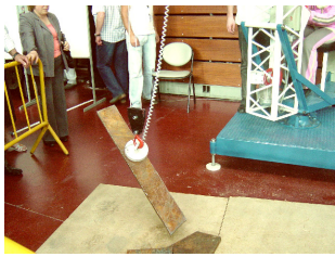
Figure 9. Electromagnet elevating an iron piece
