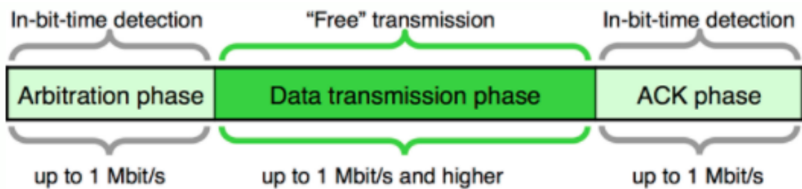
Figure 10: Illustration of the CAN FD flexible data-rate mechanism (Electronics, 2021)
