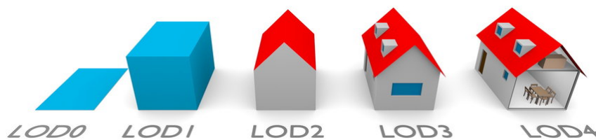
Figure 3: Different LOD levels of CityGML [8]
