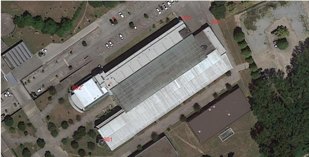
Figure 14: Four equivalent control points in the desired georeferenced location
