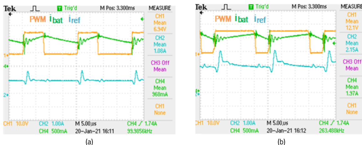
Figure 6.10: PWM signal (CH1: 10 V/div) comparison with the Load current (CH4: 500 mA/div), and the reference current (CH2: 1 A/div): (a) Results with a 1 A reference; (b) Results with a 2 A reference. Time scale of 5 \mu s/div.
