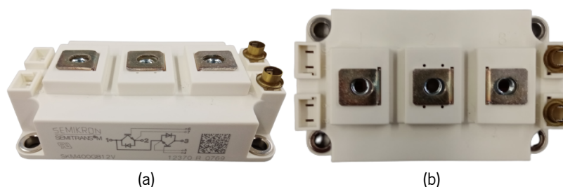
Figure 5.18: Pictures of the SKM400GB066D IGBT module: (a) Side view, showing the IGBT leg layout; (b) Top view of the IGBT.
