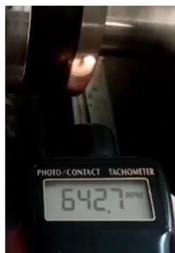
Figure 6.3: Tachometer measuring the rotation speed of the motor axle using the light emitter mode.
