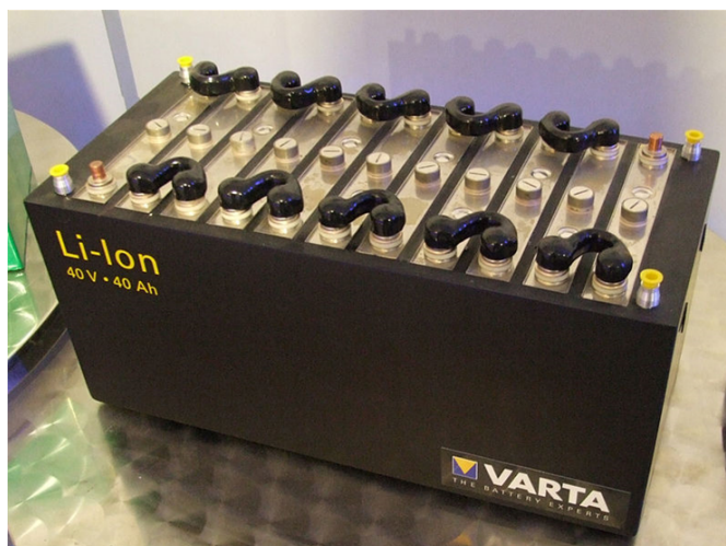
Figure 2.9: Photograph of a 1.6 kWh Li-ion battery bank produced by the company Varta. Reproduced from [39]
