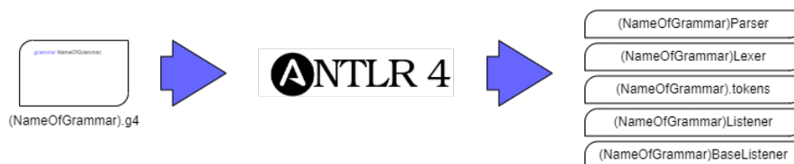
Figure 20: ANTLR creates a variety of files from the grammar.
