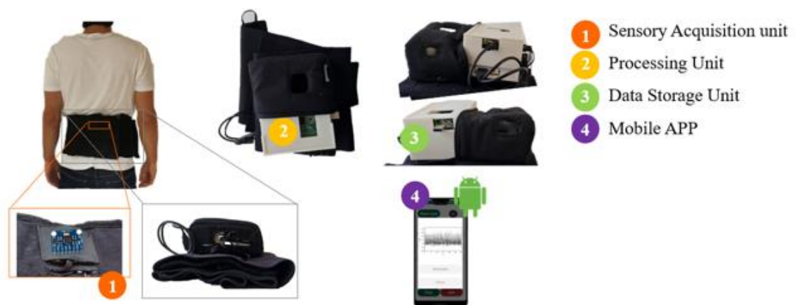
Figure 3-2 +Sense hardware and software setup.
