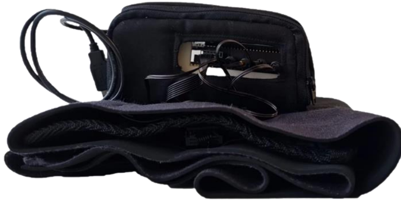
Figure 4-2 Waistband containing the MPU-6050 Inertial Measurement Unit sensor (WBD).
