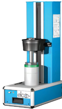
Figure 83: Utilized heat induction system, Elco's model START.2 [69].
