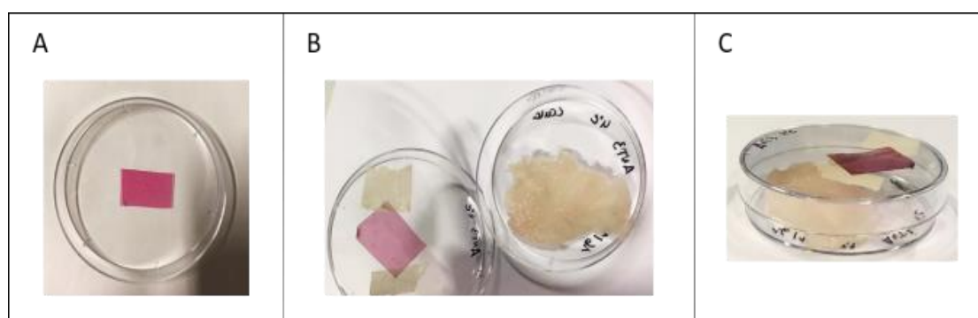
Figure 9. Illustrative example of the experimental set-up used to monitor fish freshness during storage at 4 and 25 °C. (A) Film sample (2 cm x 2 cm) fixed to Petri dish cover; (B) Petri dishes containing hake samples; (C) Closed system used for monitoring hake freshness status.
